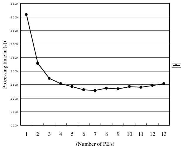
Figure 11 Relation between processing time and extent of parallel processing (without write operation of Hard Disk)
