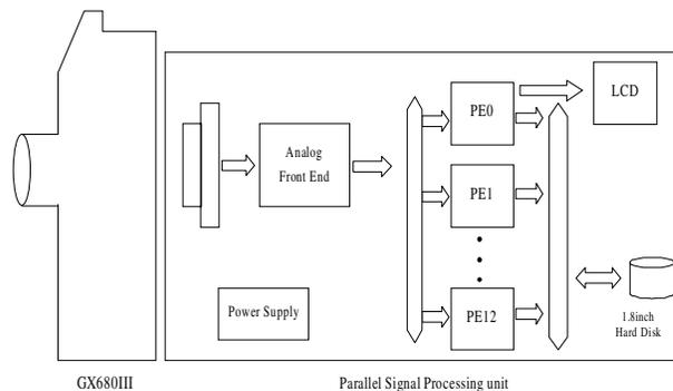
Figure 6. a block diagram of the system.
