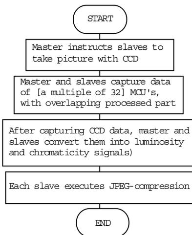
Figure 9. Signal and JPEG processing flow
