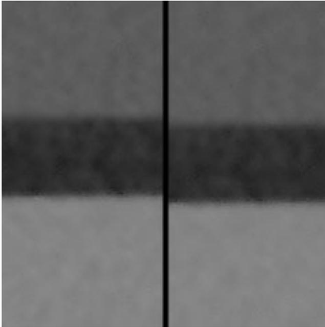
Figure 6. Example of chroma noise-reduction algorithm: (left) original, (right) noise cleaned.
