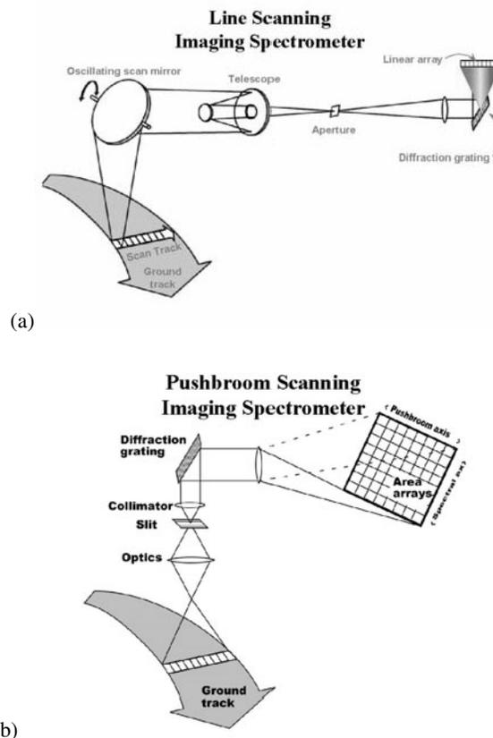
Figure 5. (a) Illustration of the line scanner and (b) push broom scanner imaging spectrometer designs.
