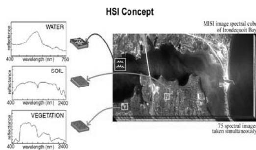
Figure 4. Illustration of the image cube concept including the concept of spectral vectors associated with each pixel. The top of the image cube shows a 3-band true color image acquired with RIT's 75 band imaging spectrometer (MISI).
