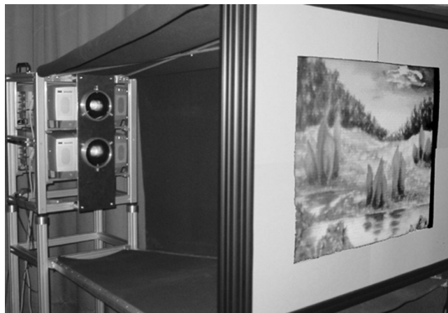
Figure 1. Laboratory model of a 6-channel display using two LCD-projectors with channels providing 50 nm narrow band spectral power distributions.
