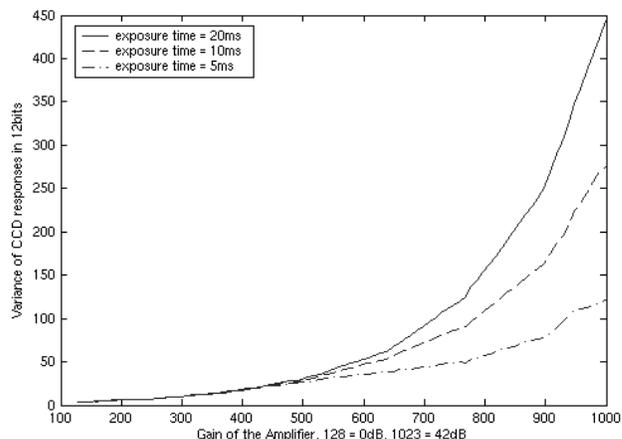
Figure 8. Standard deviation of the CCD dark noise. Each curve represents the dark noise standard deviation versus the amplifier gain obtained with a fixed exposure time. Gain is given in units accepted by the control system, 128 is 0 dB while 1023 is 42 dB.
