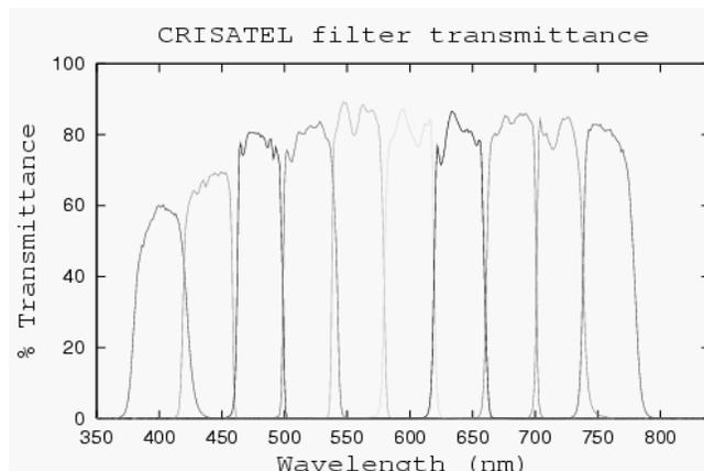
Figure 1. Transmittance of the 10 UV-VIS filters measured with the Hitachi spectrophotometer.
