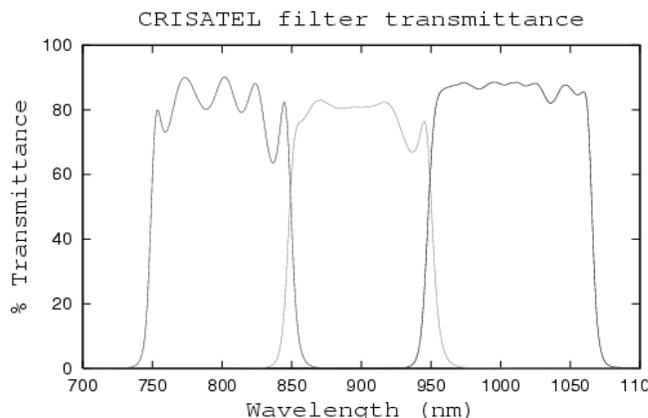
Figure 2. Transmittance of the 3 IR filters measured with the Monolight spectrophotometer
