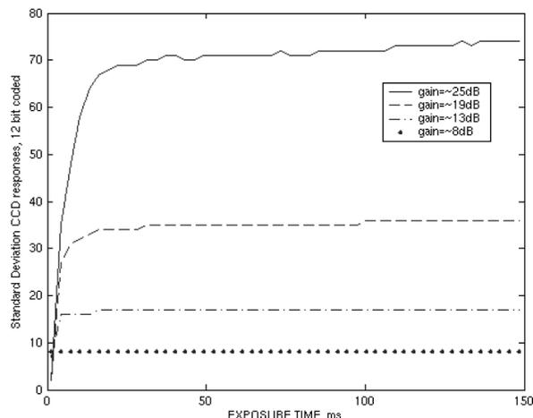
Figure 7. Standard deviation of the dark noise. Each curve represents the dark noise standard deviation versus the exposure time for a fixed amplifier gain. The standard deviation reaches a maximum which depends on the gain.
