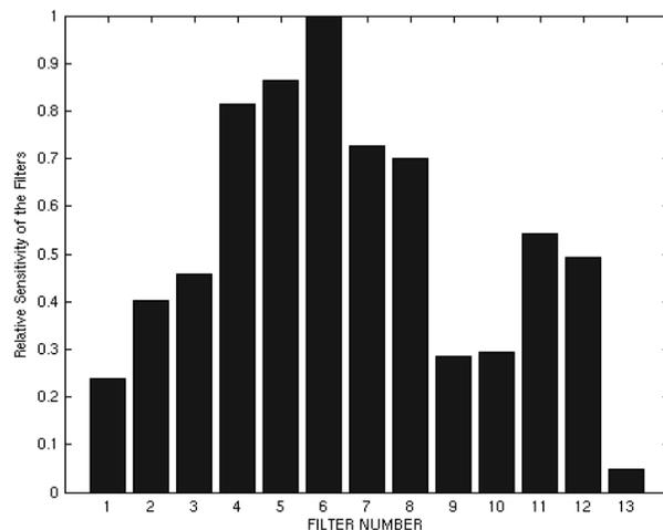
Figure 5. Relative channel sensitivity of the CRISATEL camera. Channels 1 to 10 correspond to the 10 filters in the visible spectral range, channels 11 to 13 to the three IR filters.
