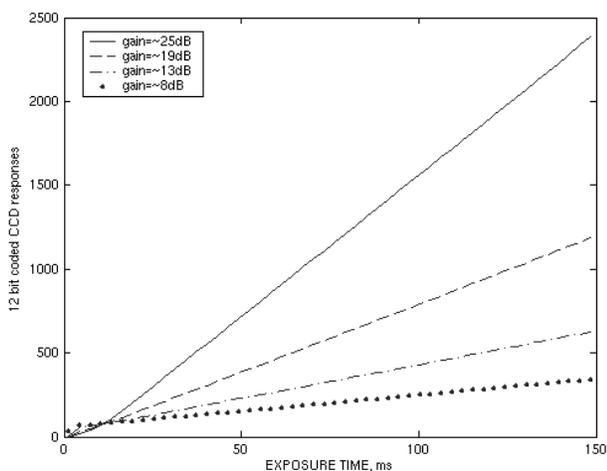
Figure 6. Mean value of the CCD dark noise. Each linear curve represents the dark noise mean value versus the exposure time for a fixed amplifier gain. The amplifier gain changes the slope of the lines.
