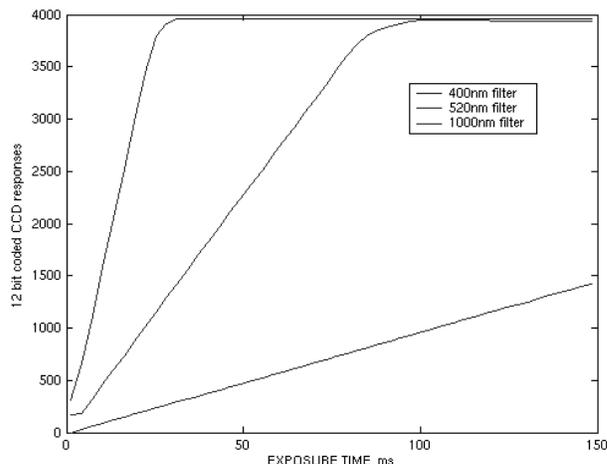
Figure 4. Curves showing the linear behavior of the CCD array for three different channels. Amplifier offset is fixed to its minimum level, amplifier gain is 0dB.
