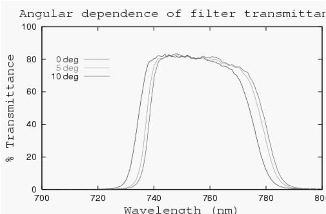
Figure 3. Angular dependence of filter transmittance.
