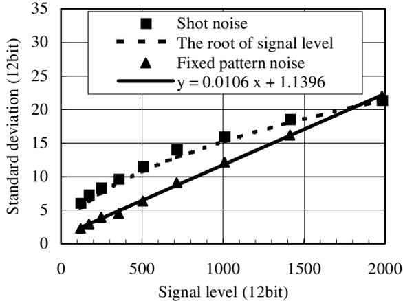
Figure 3. Properties of fixed pattern noise and shot noise
