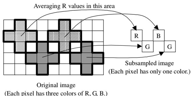
Figure 6. Subsampling pattern (In case that subsampling pitch is 2)
