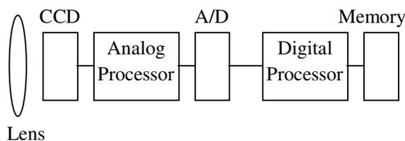
Figure 1. Structure of digital still camera
