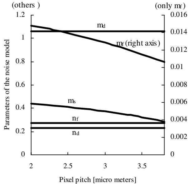
Figure 5. Parameters of the noise model with different pixel pitches
