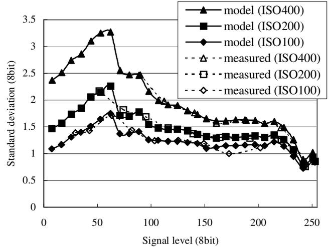
Figure 4. Correspondence between model's noise and measured noise
