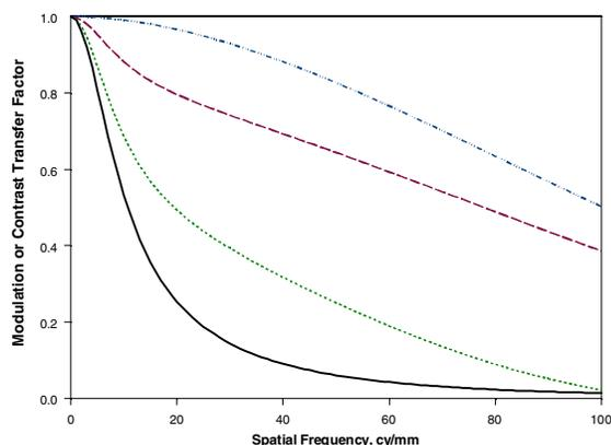
Figure 3. MTF and CTF model curves. Top curve, dot-dash is the emulsion layer MTF, next lowest curve, dashed is the photographic paper exposure MTF, the dotted curve is the paper CTF, and the bottom, solid, curve is the paper substrate MTF.
