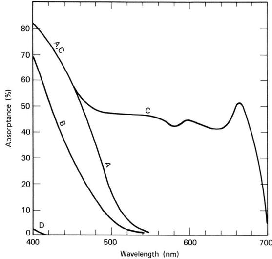
Figure 1. Absorbance spectra for several different silver halide emulsions. A = undyed negative type, B = extremely fined grain type, C = A with sensitizing dye, and D = pure silver chloride. From Ref. (26)
