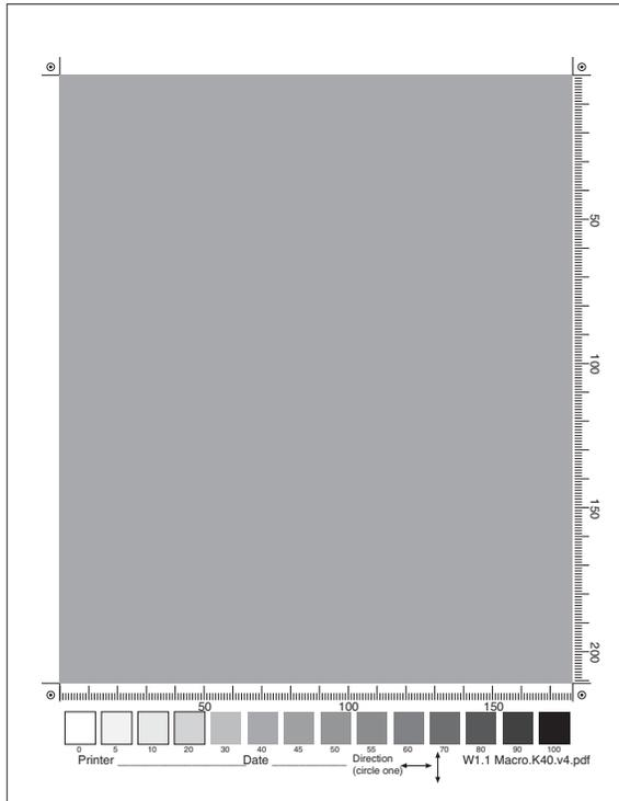
Figure 1. The “W1.1.Macro.K40” (version 4) test pattern, reduced to approximately 35% size.
