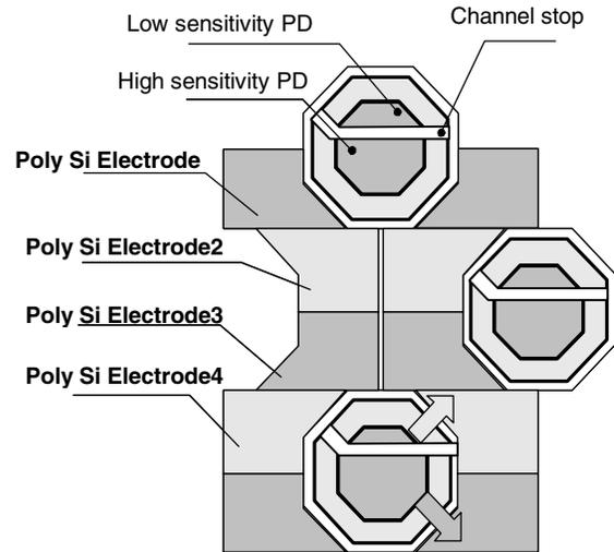
Figure 5. The layout of photodiodes and electrodes
