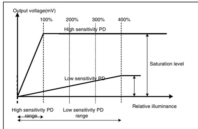
Figure 6. The relationships between relative illuminance and relative output voltages
