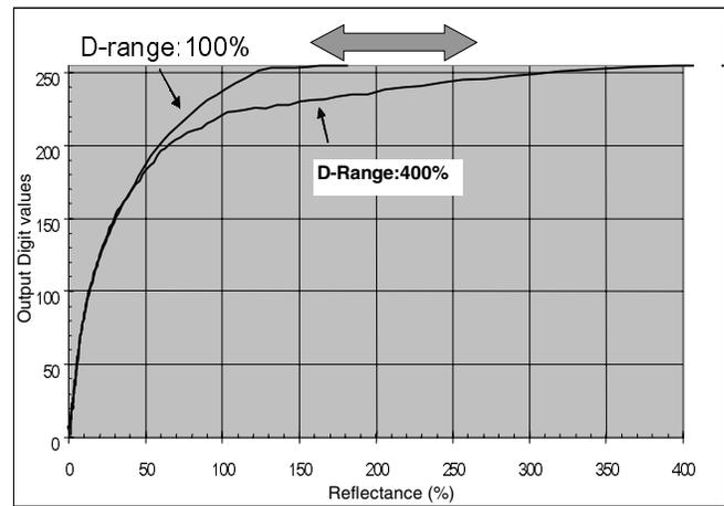
Figure 8. Opto-electronic conversion functions for combined images. Two examples, in case of 100% and 400%, are shown in the figure.
