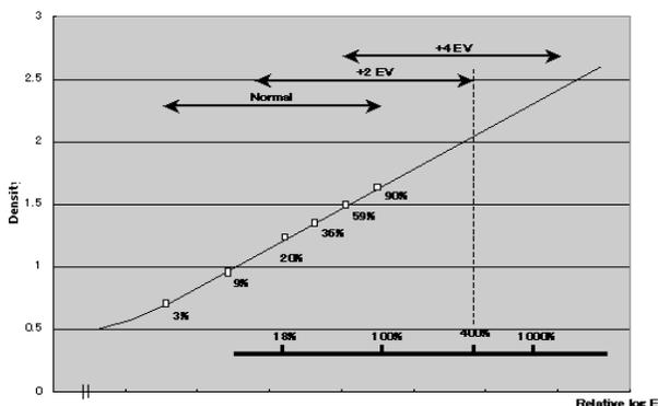
Figure 2. Characteristic curve of the green sensitive layer of typical negative film and its dynamic range
