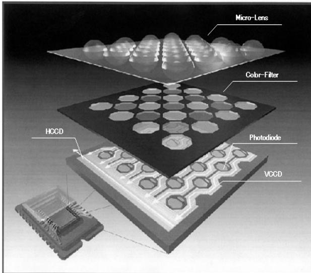
Figure 4. Sketch of a newly developed CCD
