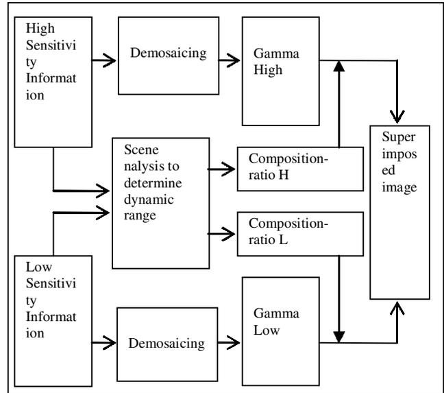
Figure 7. The flow of the algorithm to build up a final image
