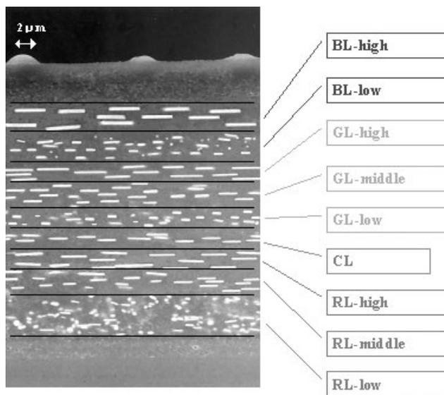
Figure 3. Cross section of a color negative film
