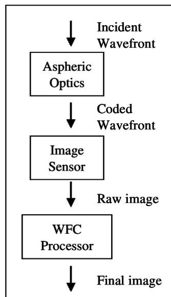
*Figure 1. System block diagram. Specialized optics produce images that are insensitive to misfocus like aberrations. A blurred “raw” image is digitized at the detector. Processing of the digital blurred image produces a sharp final image free of aberrations.*
