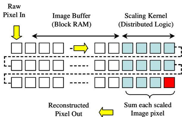
Figure 4. Block diagram of the basic convolution algorithm. Buffers are used for delay-line structures. The taps perform scaling on the input pixel values and an adder provides the final tap output.
