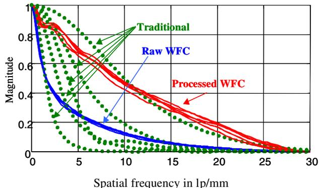
Figure 3. MTFs as a function of misfocus. Traditional system drastically loses spatial resolution with misfocus. Wavefront Coded MTFs before signal processing are lower than the in-focus traditional system but essentially constant with misfocus. After signal processing all Wavefront Coded MTFs are very similar to the in-focus one.
