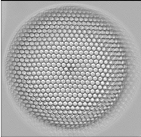
Figure 7. Wavefront Coded microscope image, reconstructed at 30 frames/second with a 17x17 sized kernel. Note the clear depth of focus extension in the Wavefront Coded image. The depth extension is approximately 2 to 4 times.
