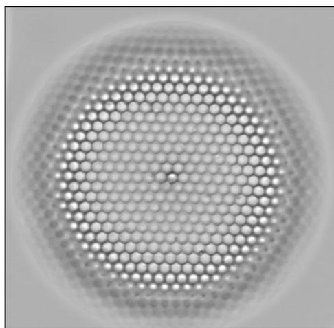
Figure 6. Traditional microscope image. Only an annular region with a thickness of about  $1/4$  the radius of the object is in focus. The in-focus annulus is the ring of highest contrast, roughly centered between the middle of the object and its edge.
