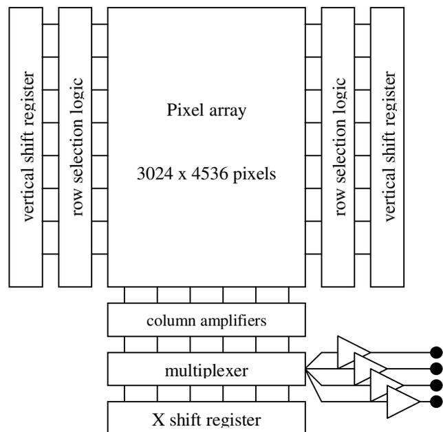
Figure 4. Architecture of the image sensor
