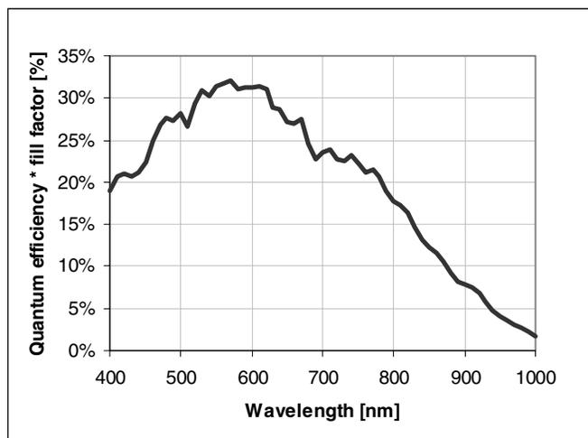
Figure 5. Quantum efficiency  $\times$  fill factor (monochrome sensor without cover glass)
