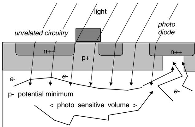
Figure 3. Principle of high-fill factor pixel
