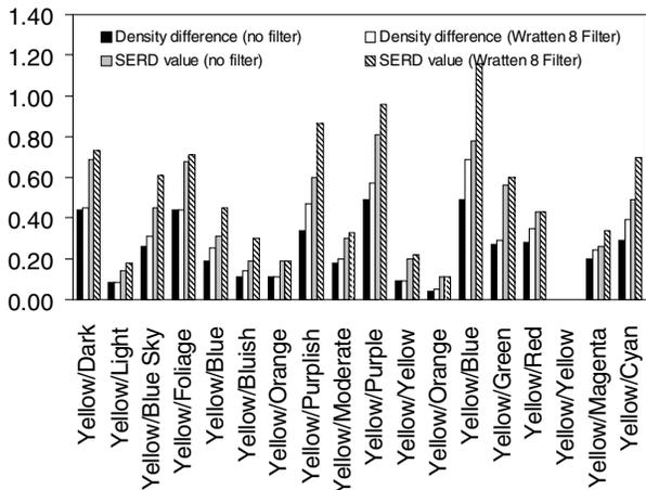
Figure 3. Density differences and SERD values for yellow patch relative other colour patches of the Macbeth ColorChecker Chart, recorded on Ilford FP4 film with and without filtration.
