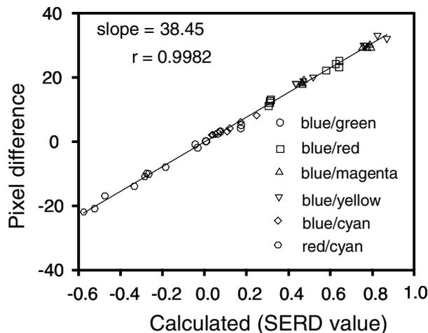
Figure 5. Measured mean pixel value differences vs calculated SERD values of the indicated patches of the Macbeth ColorChecker Chart for the CCD system.
