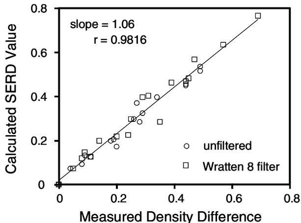
Figure 4. Measured density differences vs calculated SERD values of yellow patches relative to all other colour patches of the Macbeth ColorChecker Chart for the photographic system.
