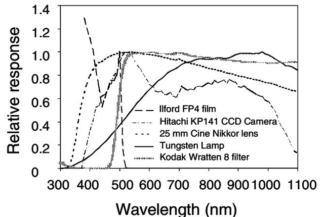
Figure 2. Spectral data for various components of the imaging chain.
