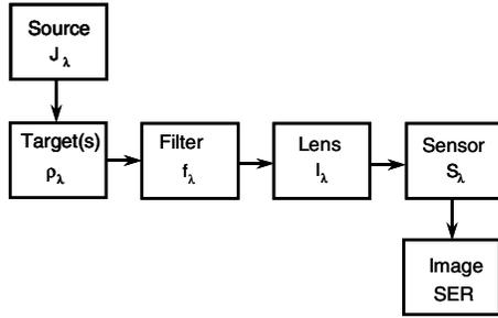
Figure 1. The imaging chain.  $SER$  = system exposure response.
