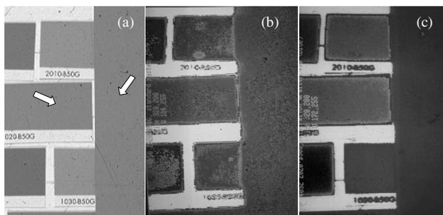
Figure 9. Monochrome versions of two visually identical paint samples indicated by the white arrows. The left hand arrow ICI Dulux 20220-B50G and the right hand arrow NCS register 2020-B50G. (a) Failure to differentiate targets by direct CCD image capture, (b) Failure to differentiate after image processing, (c) successful differentiation using a blue filter suggested by the SERD calculation.
