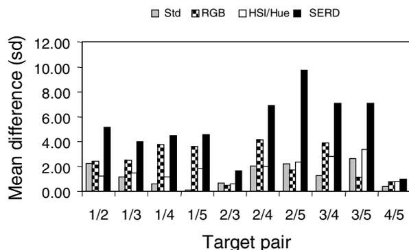
Figure 10. Mean pixel value differences as standard deviations for sample pairs. Std = standard unfiltered image capture system. RGB = optimised principal components transform applied to RGB image. HSI/Hue = hue channel of HSI transformed image. SERD = system filtered according to results of SERD calculation.
