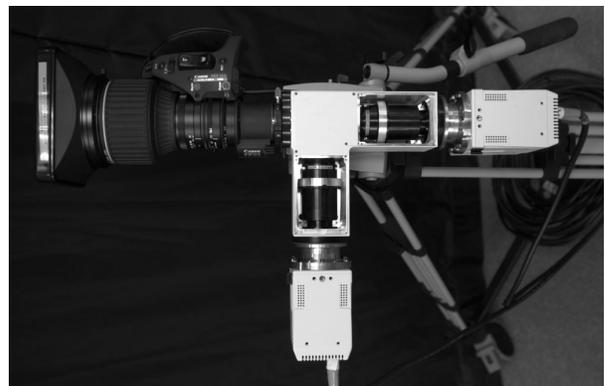
Figure 4. The 6-band separation filter location in the 6-band camera
