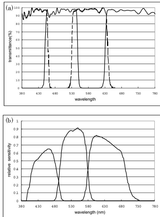
Figure 3. Spectral characteristics (a) Spectral transmittance of 6-band separation filters (b) Spectral sensitivities of the HDTV camera
