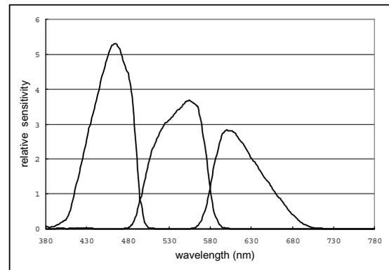
Figure 5 (b). Spectral sensitivities of the RGB camera
