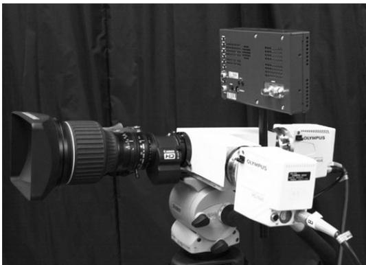
Figure 1. 6-band HDTV camera
