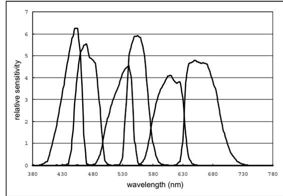
Figure 5 (a). Spectral sensitivities of the 6-band camera
