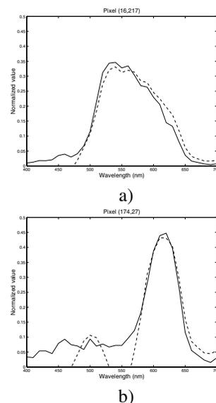
Figure 12: Spectra at two different locations of the spectral image. Solid lines: 31 interference filters, dashed lines: reconstructed from the spectral synthesizer based system data.
