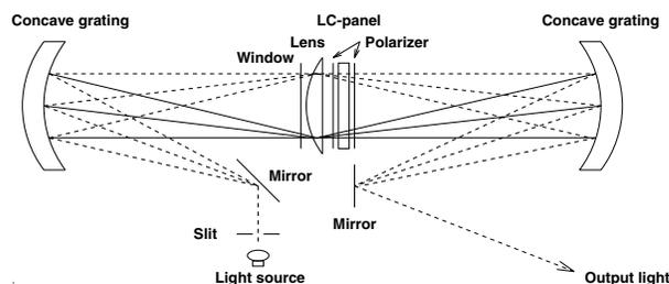
Figure 2: Optical setup for the spectral synthesizer.
