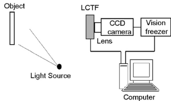
Figure 8: Experimental setup for LCTF based system.
