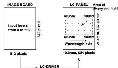
Figure 3: Schematic drawing of control of the LC-panel.
