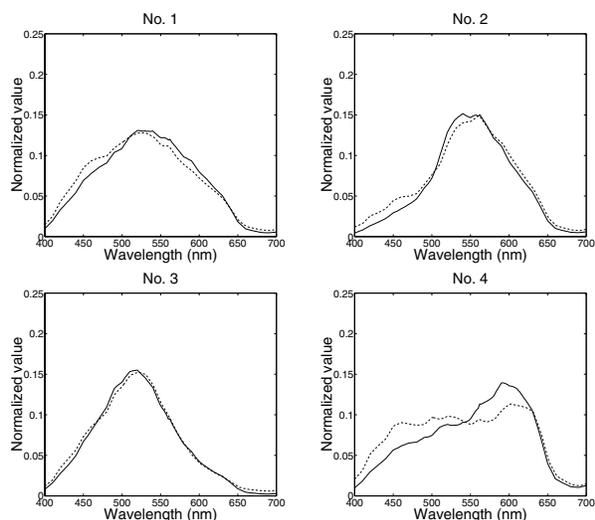
Figure 10: Optically measured results of the filtered illuminator. Solid lines are designed color filters multiplied by the light source spectrum and dotted lines are measured results.
