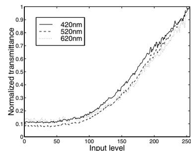
Figure 4: Spectral characteristics of the LC-panel.
