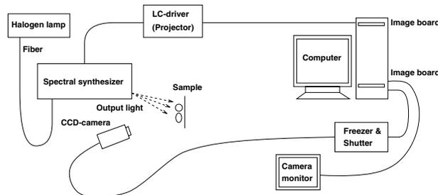
Figure 5: Spectral image acquisition system.
