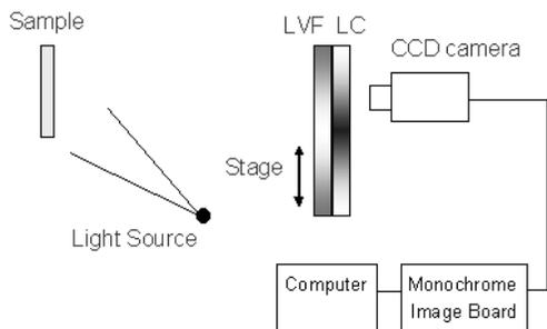
Figure 6: Experimental setup for LVF-LCSLM based system.
