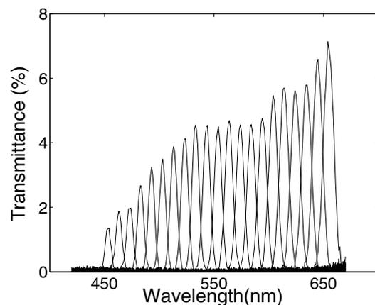
Figure 9: The transmittances of the LCTF measured for every 10-nm interval.
