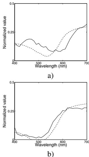
Figure 14: Spectra at two different locations of the spectral image. Solid lines: 31 interference filters, dashed lines: reconstructed from the LVF-LCSLM based system data.
