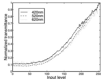
Figure 4: Spectral characteristics of the LC-panel.
