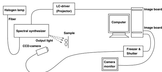
Figure 5: Spectral image acquisition system.
