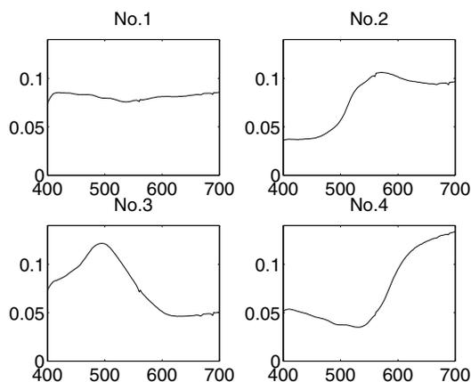
Figure 1: Designed filters for the Munsell spectral database.
