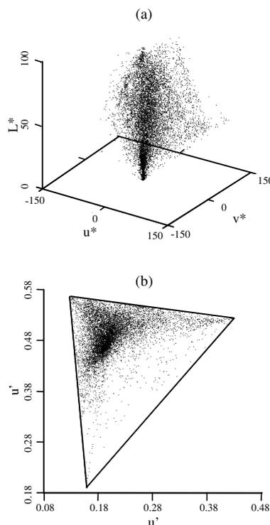
Figure 1. A random sample of the color statistics of 630 natural images in the CIE (a)  $L^*u^*v^*$  color space, and (b)  $u'v'$  diagram. The solid line indicates the PAL TV color gamut.
