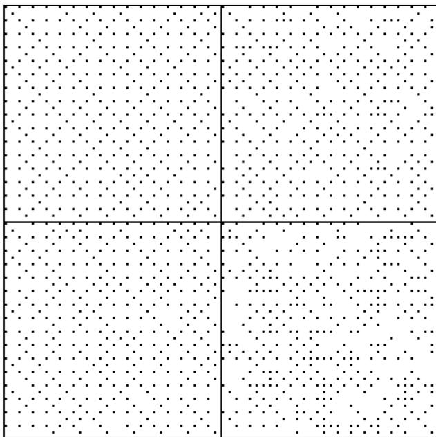
Figure 4. Adding noise to the dot order can break up the patterns caused by recursive tessellation. A first method of adding noise is here applied for different parameters. For the upper row  $p_{\text{swap}} = 0.1$ . For the bottom row  $p_{\text{swap}} = 0.5$ . The maximum swap distance is 50 for the left column and 200 for the right column.
