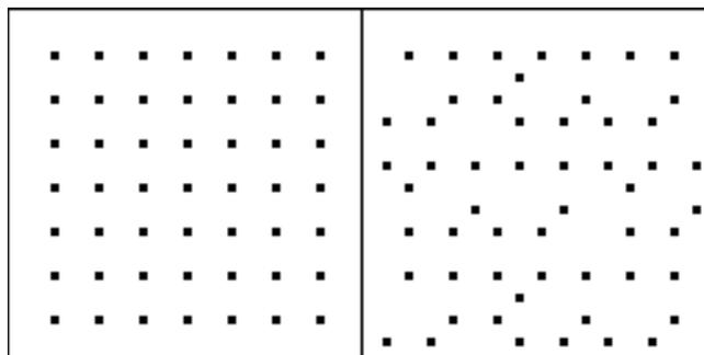
Figure 2. The pattern caused by AM-dot withdrawal also depends on the size of the tile. The left image is rendered with a tile that contains 4 by 4 AM-dots. The tile of the right image contains 5 by 5 periods. For the second tile recursive tessellation is not possible.
