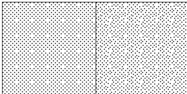
Figure 6. When only a few AM-dots are withdrawn the empty spaces become very visible when the tile is repeated. Adding positional noise can make the pattern more pleasing.
