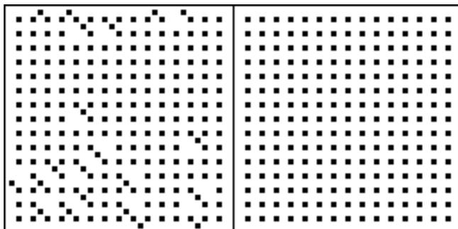
Figure 1: Classical void finding filter with fixed  $\sigma = 1.5$  x period doesn't work for large tiles as can be seen in the left image. A second algorithm to determine the dot order will give the correct recursive tessellation order (right tile).
