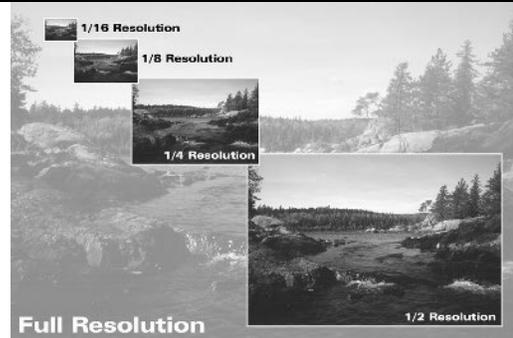
Figure 5. Resolution progressive decoding
