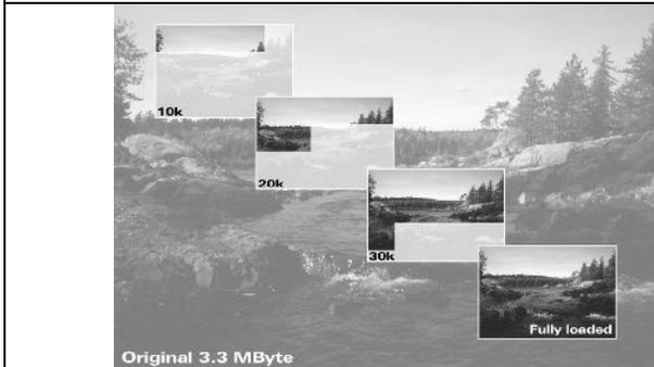
Figure 6. Position progressive decoding
