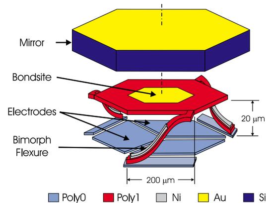
Figure 2. Tip, tilt and piston micro-mirror.<sup>2</sup>
