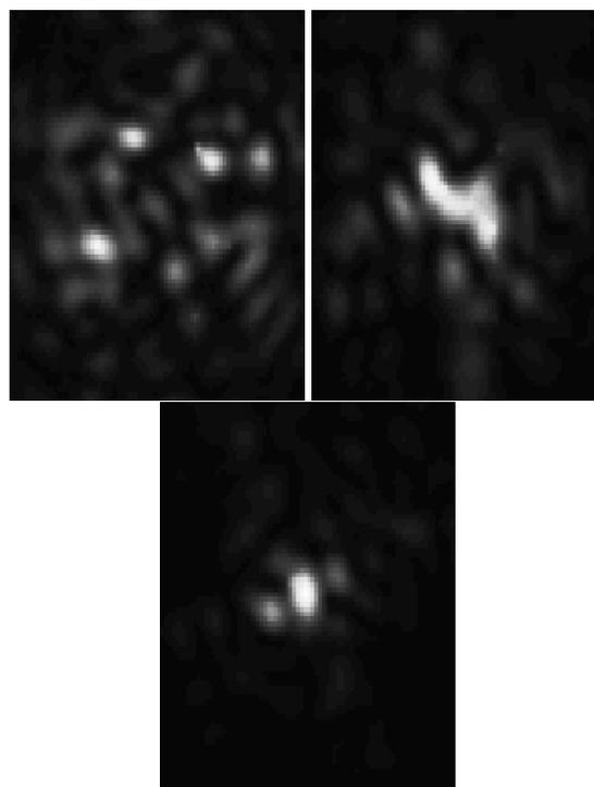
Figure 5. Intensity distribution in the confocal image plane. Top left: no AO. Top right: with AO, simple wavefront sensing. Lower: with AO, intensity weighted wavefront sensing
