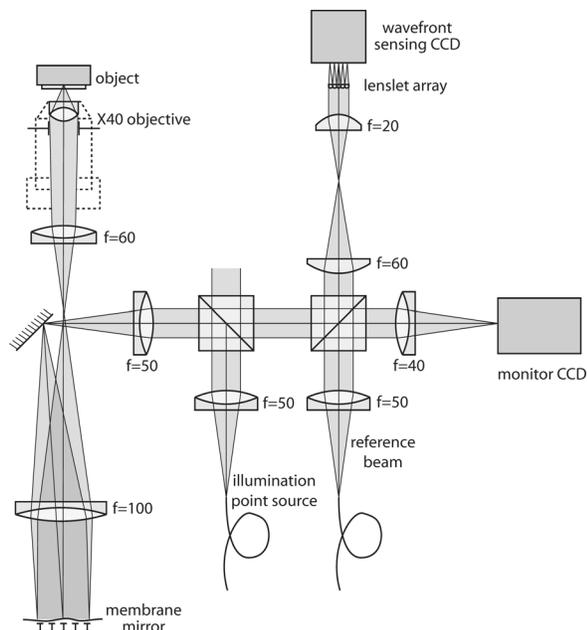
Figure 4. Schematic layout of a confocal microscope breadboard using adaptive optics
