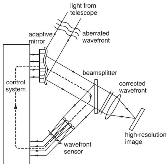
Figure 1. Schematic of an adaptive optics system for astronomy
