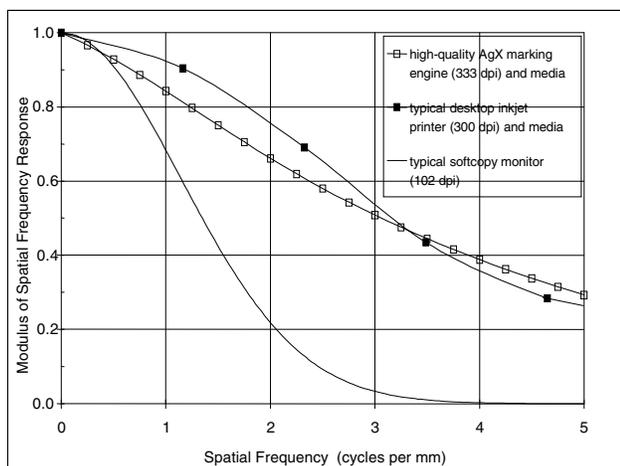
Figure 1. The MTFs of three device-media combinations.
