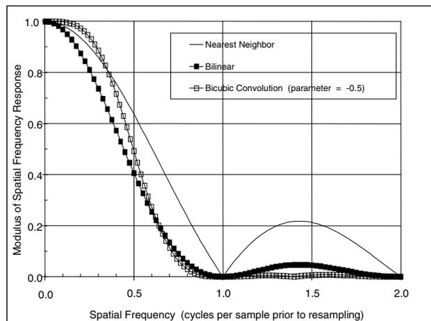
Figure 2. The phase-averaged MTFs of three common resampling techniques.<sup>18</sup>
