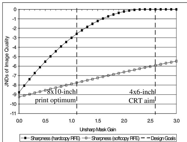
Figure 4. The effect of spatial filter gain level on the perceived sharpness of a particular 3.1-mega-pixel DSC capture written to 8 x 10-inch reflection media at 333-dpi and displayed at 4 x 6-inch size on an 102-dpi CRT monitor.
