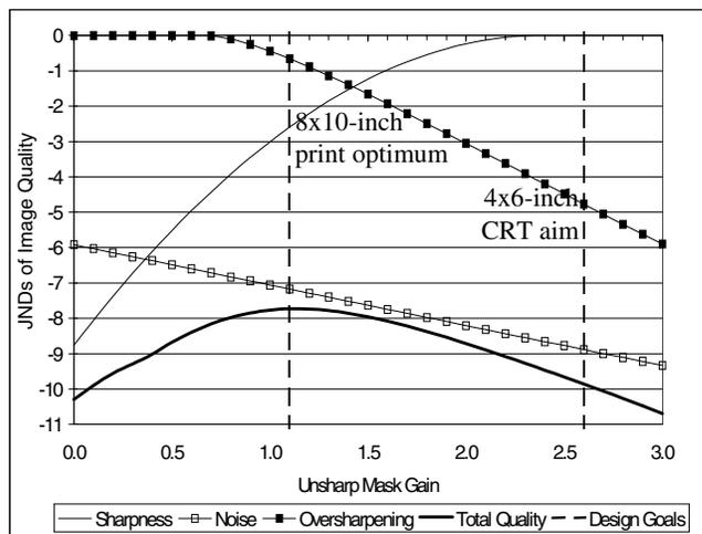
Figure 3. The effect of spatial filter gain level on the quality attributes of a particular 3.1-mega-pixel DSC capture written to 8 x 10-inch reflection media at 333-dpi.
