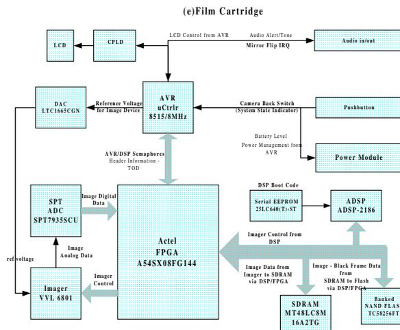
Figure 3. – (e)film detailed block/functional diagram
