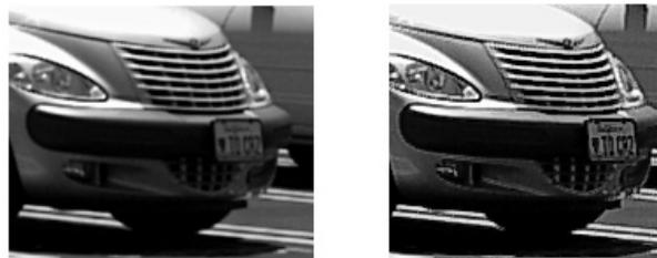
Figure 4. Left image: anti-aliasing & sharpening disabled; Right image: anti-aliasing and sharpening enabled
