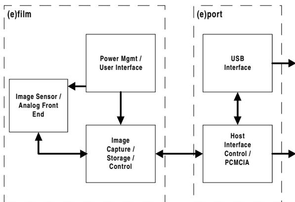
Figure 2. Functional Block Diagram of (e)film and (e)port
