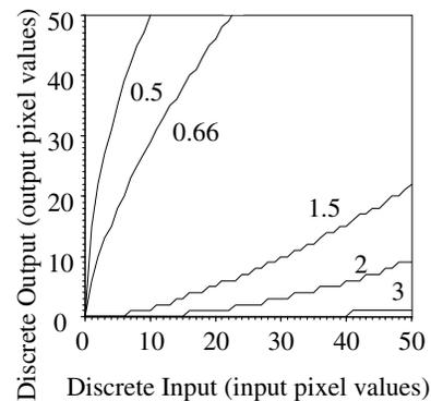
Figure 1. Stepping introduced to the gamma corrected signal due to the use of integer mathematics for the values of gamma correction shown.
