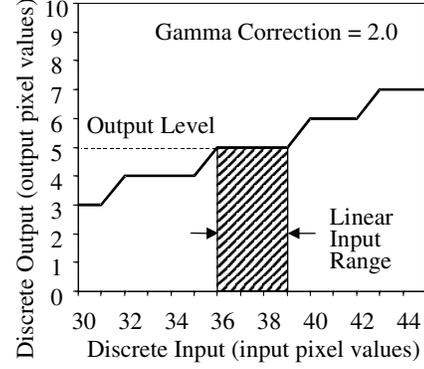
Figure 2. A magnified portion of a gamma corrected signal showing the ambiguity caused when linearizing a digital signal. The output value of 5 is mapped to input pixel values of 36 to 39.
