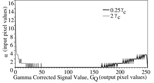
Figure 3. A graph of the numerical range of input values,  $\alpha$ , versus gamma corrected signal values.
