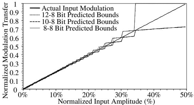
Figure 8. Predicted modulation range for a signal gamma corrected with a value of  $\gamma_c=3$ . The curves show the effect of changing input bitdepth. Both target and acquisition gamma is assumed to be unity. The output bitdepth is 8 bits.
