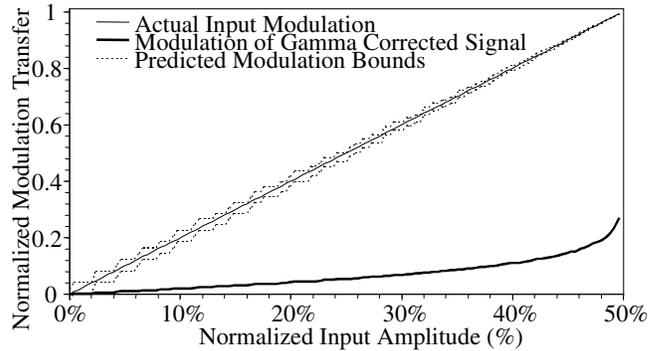
Figure 6. The predicted modulation range for a signal with gamma correction of 0.1 applied. The input and output bitdepth is 8 bits.
