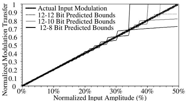
Figure 9. As for Figure 11, though changing the output bitdepth. The input bitdepth is 12 bits.
