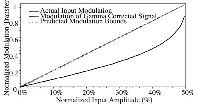
Figure 4. Predicted modulation range for a signal with gamma correction of 0.45 applied. The input and output bitdepths are both 8 bits.
