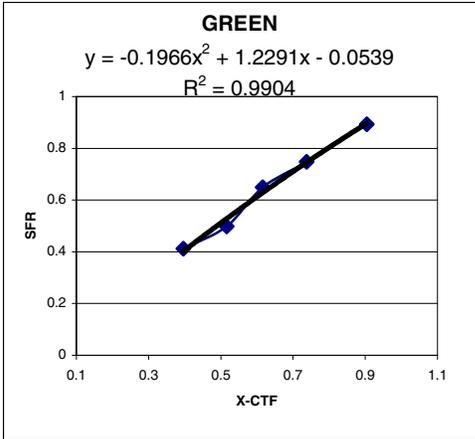
Figure 7. SFR versus CTF for the green channel @ 1200ppi with medium sharpening.
