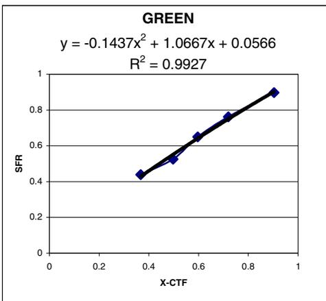
Figure 8. SFR versus CTF for the green channel @ 600ppi with no sharpening.
