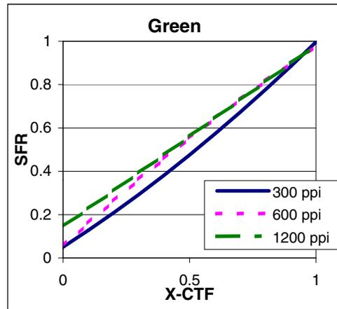
Figure 10. Curves obtained from 300, 600 and 1200 ppi with no sharpening, SFR versus CTF comparison for a one scanner.
