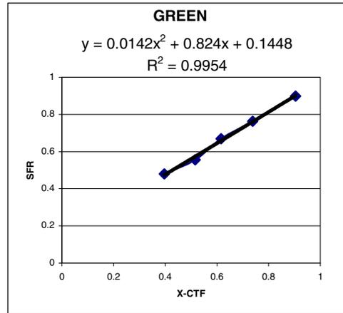
Figure 9. SFR versus CTF for the green channel @ 1200ppi with no sharpening.
