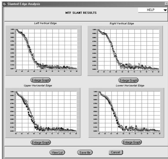
Figure 4. Output of SFR executable file displaying 4 outputs of the 4 slanted edges.
