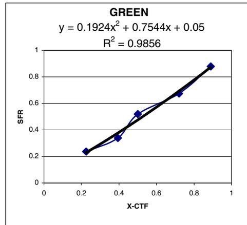
Figure 6. SFR versus CTF @ 300ppi with no sharpening applied.
