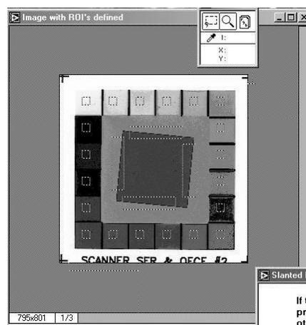
Figure 3. SFR scanner target with ROIs and gray scale selected.
