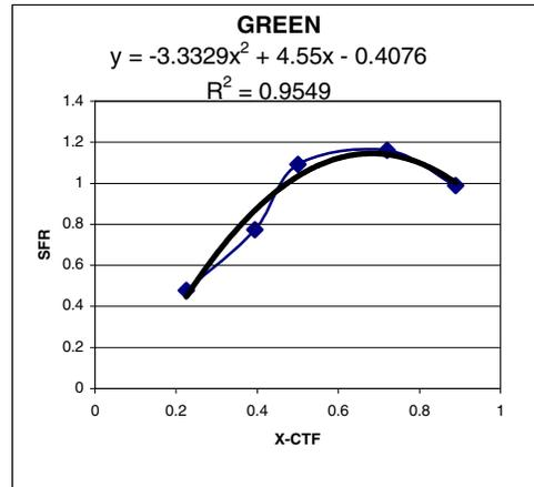
Figure 5. SFR versus CTF @ 300ppi with extreme sharpening applied.
