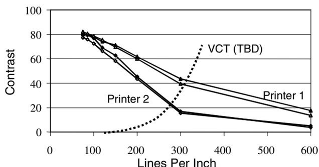
Figure 4. Measured Contrast for Two Printers
