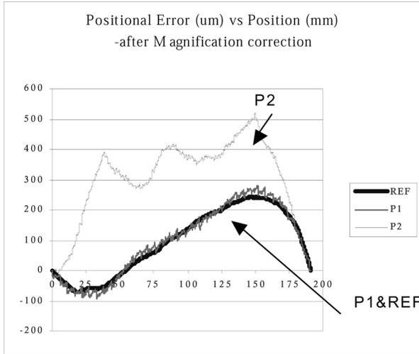
Figure 3. Positional error result after correction for magnification.
