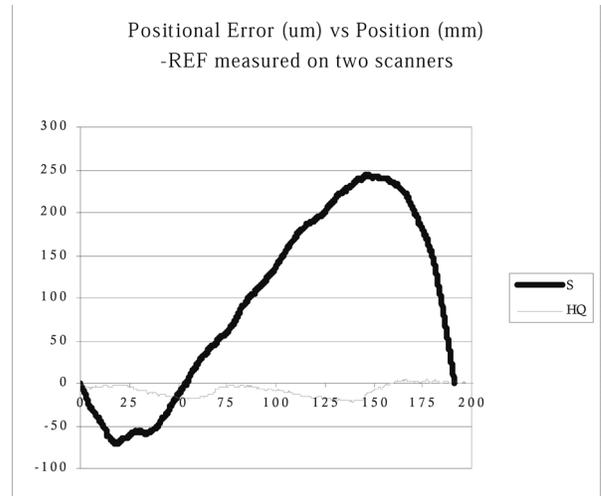
Figure 4. Positional error for REF target measured on test scanner (S) and very high quality scanner (HQ).
