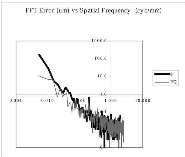
Figure 7. Spectral results for REF image measured on test scanner (S) and High Quality Scanner (HQ).
