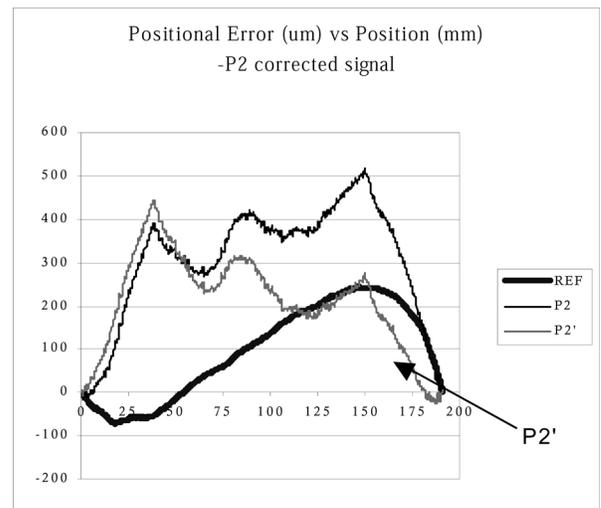
Figure 6. Positional error of P2 before and after correction
