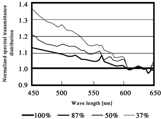
Figure 10. Normalized spectral transmittance distribution of the LC panel corresponds to digital code value.
