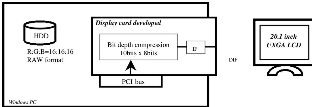
Figure 8. Schematic diagram of the high bits depth LCD imaging system
