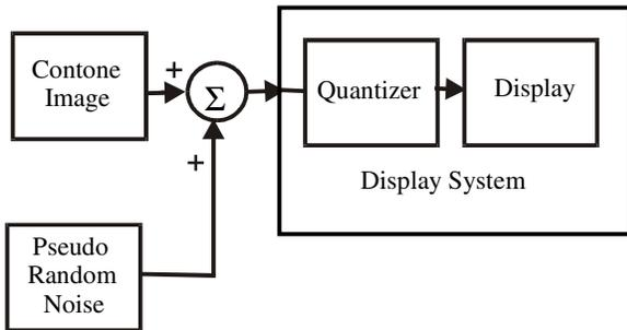
Figure 7. Basic application of Robert's noise modulation to displays
