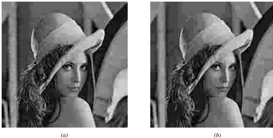
Figure 4. Blocking artifacts resulting from different algorithms, (a) improved algorithm requiring 0.28 bit/pixel, (b) standard JPEG algorithm requiring 0.31bit/pixel.
