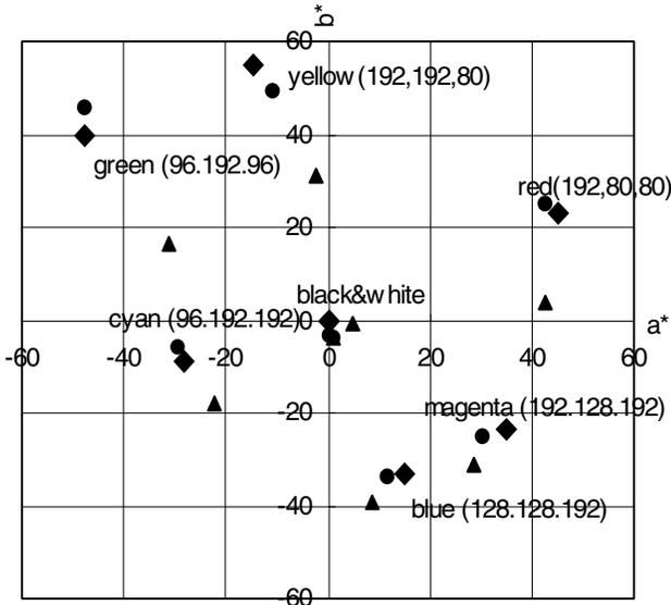
Figure 7. Effects of compensation by the use of ICC profile. Compensation is shown as chromaticity points on a\*b\* diagram. Triangle mark(Δ ):LCD display original(measured); Circle mark(○):with the ICC profile(measured); Diamond shape mark(◊) :sRGB standard(calculated)
