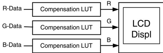
Figure 3. Schematic diagram of compensation on display data model
