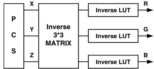
Figure 4. Schematic diagram of color processing model for displays
