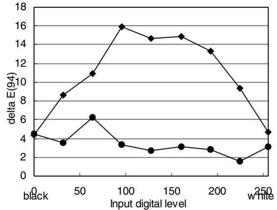
Figure 8. Delta E(94) varying the input digital level for gray patches. References are gray for sRGB. Circle mark(○) : with the ICC profile(measured); Diamond shape mark(◊): without the ICC profile(measured)
