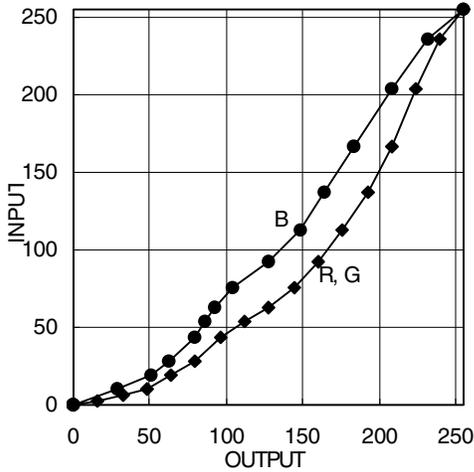
Figure 6. Inverse LUTs compensating the color reproduction on ICC profile. R: LUT for red data. G: LUT for green data, B: LUT for blue data.
