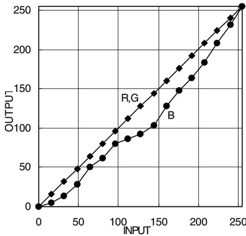
Figure 2. Compensation LUTs for an LCD.
