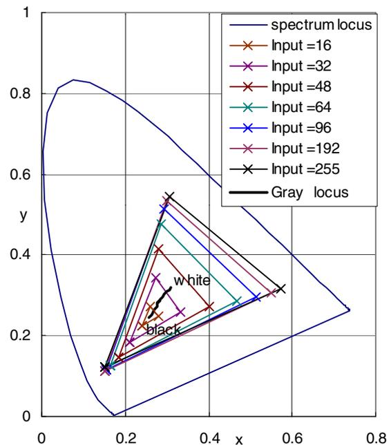
Figure 1. Color gamuts of an LCD varying the input digital level. Measurements were made by using 8 bits RGB inputs. "Input=16" indicates the gamut for  $R(16,0,0)$ ,  $G(0,16,0)$ ,  $B(0,0,16)$ . "Input=255" indicates the gamut for  $R(255,0,0)$ ,  $G(0,255,0)$ ,  $B(0,0,255)$ . "Gray locus" shows the locus for varying the gray inputs from white(255,255,255) to black(0,0,0).
