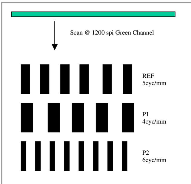
*Figure 1. Illustration of samples and scan orientation. The scanner output is a 1200 spi (8-bit) grayscale TIFF image*
