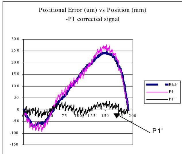
Figure 5. Positional error of P1 relative to REF.
