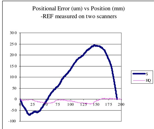
Figure 4. REF target error measured on 2 scanners; nominal(S) and very high quality scanner (HQ).
