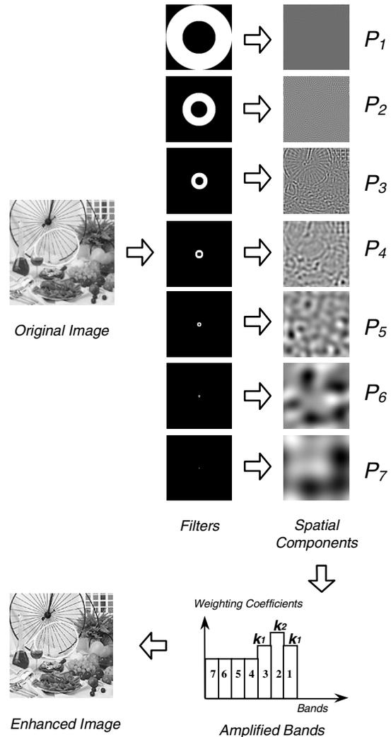
Figure 2. Ensemble of filters and weighting functions.
