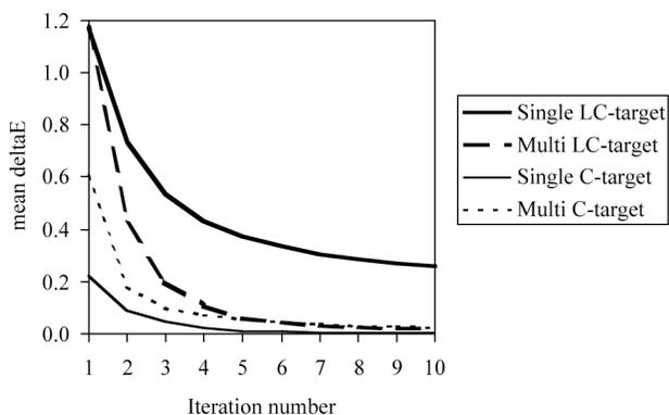
Figure 1. Mean colour difference ( $\Delta E_{97s2}$ ) between histogram-match image and gamut-mapped images obtained using different target histograms in the HEC approach.
