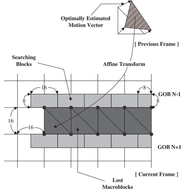
Figure 1: Error concealment method using affine transform.
