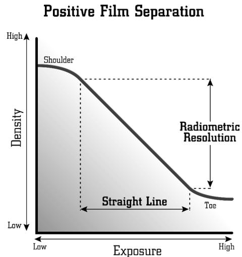
Figure 2. *Requisite sensitometry. Fitting the radiometric resolution of the imaging system into the range of densities in the straight-line portion of a film separation's sensitometric curve assures an even and equitable progression of density steps that regulate color exposure.*
