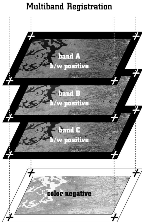
Figure 3. Multiband registration. The crosshairs in each corner of the film separations occupy the same pixel address among all three black-and-white positive records. Their accurate registration assures a controlled composite in the first generation color negative.
