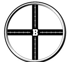
Figure 4. Comparative pixel measurements. The functional integrity of a color signature is based on the comparative measurements of the biaxial dimensions of a pixel in a film separation with a corresponding pixel in the color negative. That pixel is located at the intersection of the crosshairs in each corner of the positive and negative.
