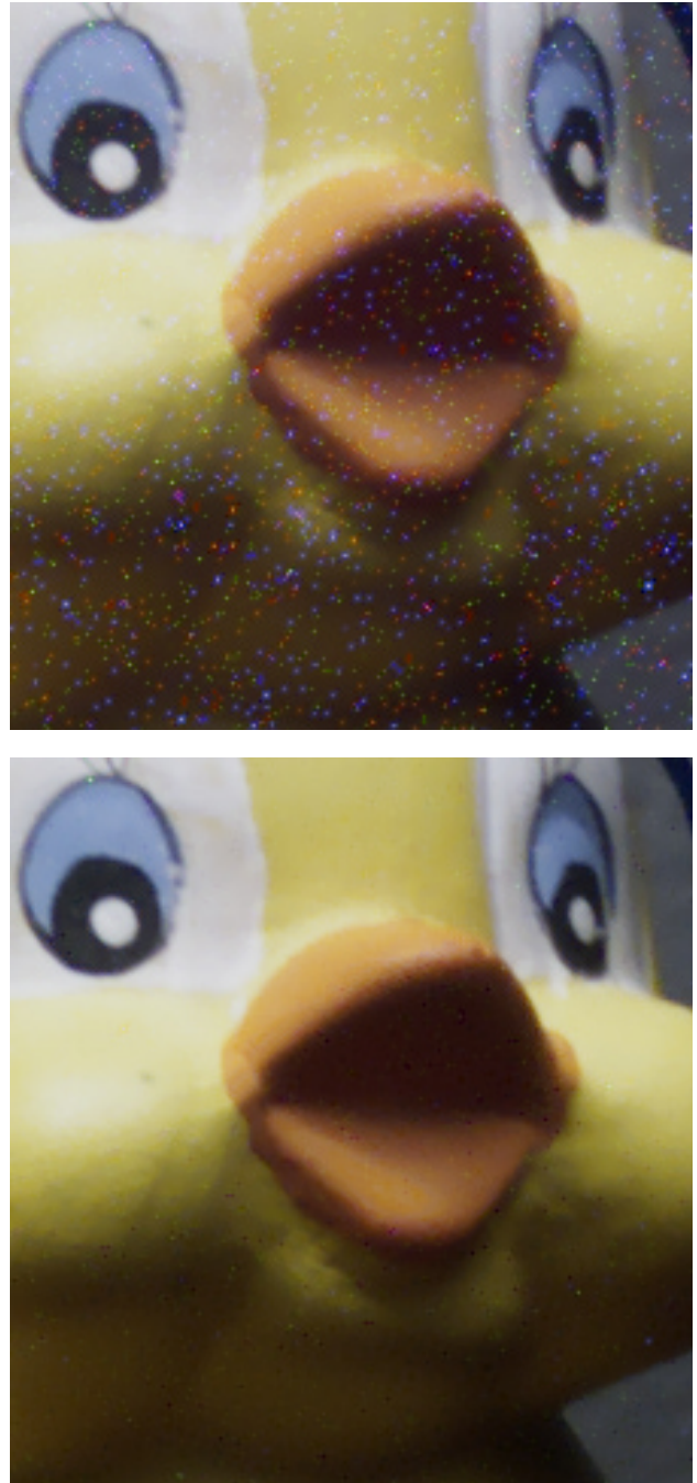
Figure 4: Color images taken from test image B. The upper version was not corrected, the lower image was corrected using our method. The images were reconstructed using the threshold-based variable number of gradients method [2].
