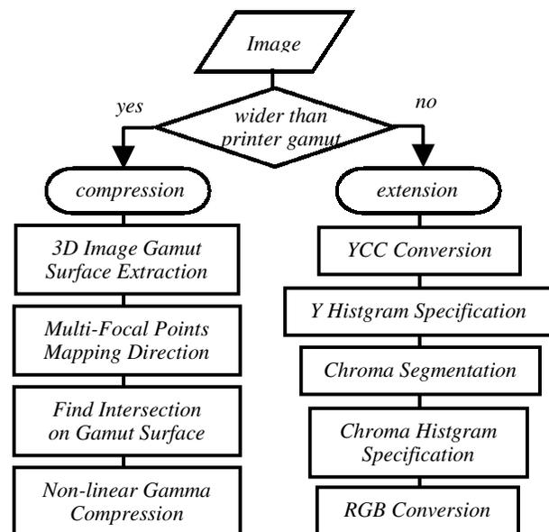
Figure 2. Diagram of proposed gamut mapping system
