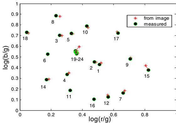
Figure 2. Chromaticity diagram showing more accurate prediction of image colors calculated from measured data. (Asterisks are chromaticities calculated from digital camera image data and dots are chromaticities predicted from measurements of light reflected off surfaces and camera spectral sensitivities.)
