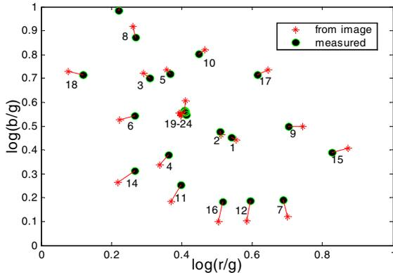
Figure 1. Chromaticity diagram showing desaturation of the more saturated colors caused by crosstalk in camera system. (Asterisks are chromaticities calculated from digital camera image data and dots are chromaticities predicted from measurements of light reflected off surfaces and camera spectral sensitivities.)
