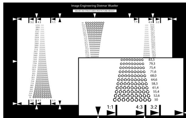
Figure 9. Circular structures for visual resolution evaluation
