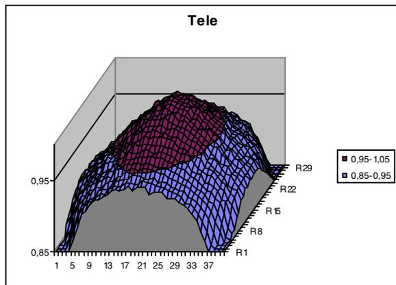
Figure 10. Shading of Fuji Finepix 4900 (normalized values)
