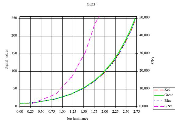
Figure 1. OECF daylight of Leica S1 with high dynamic range
