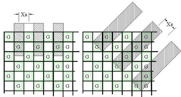
Figure 15. green array line pairs at the Nyquist frequency
