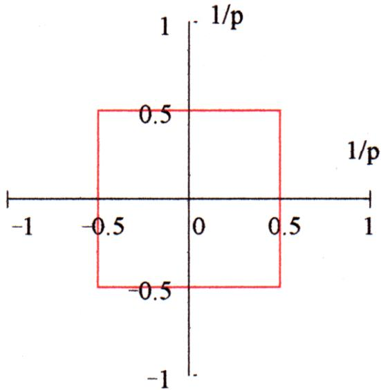
Figure 10. Nyquist domain graph, units of cycles/unit length. Normalized to the sampling frequency
