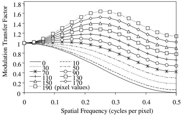
Figure 4. MTF with respect to edge contrast for a system with non-linear sharpening.
