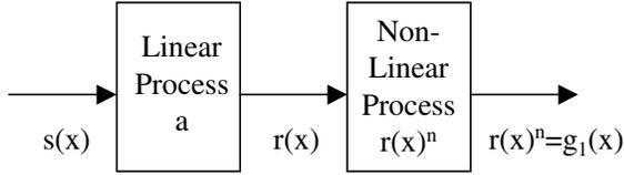
Figure 7. A non-linear system comprising of linear and non-linear components.
