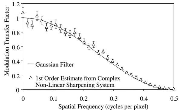
Figure 11. First order magnitude estimate for the system with the complex non-linear sharpening filter.
