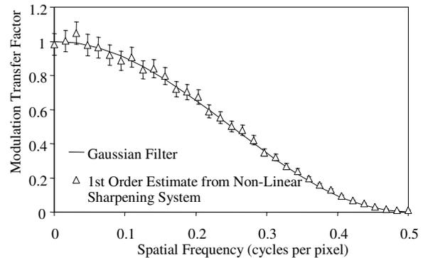
Figure 10. First order magnitude estimate for the system with the non-linear sharpening filter.
