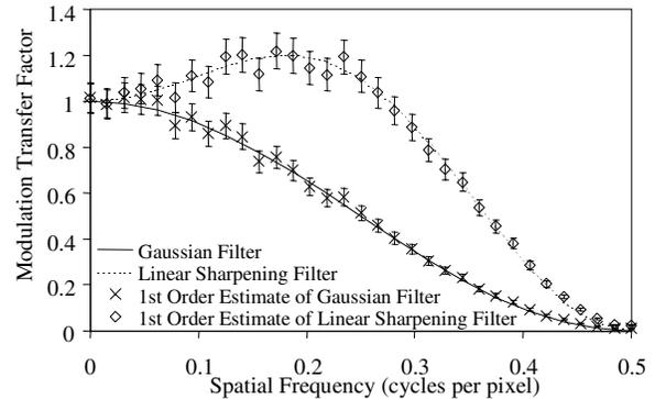
Figure 9. Magnitude estimate of the first order Wiener kernel transforms for the Gaussian filter and linear sharpening filter.
