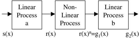
Figure 8. An LNL system comprising a non-linear component 'sandwiched' between linear parts.
