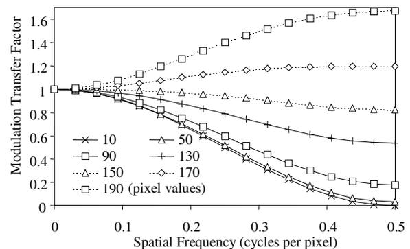
Figure 1. MTF of a system with non-linear sharpening. Each curve represents a test edge of differing magnitude.
