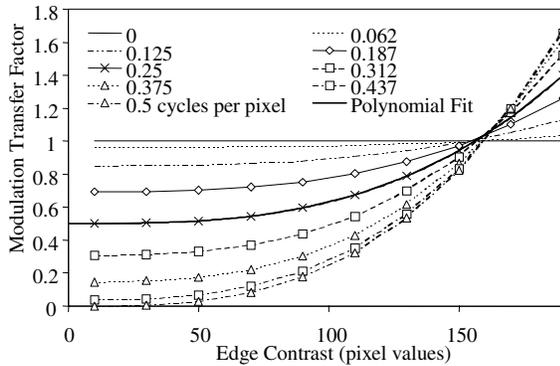
Figure 2. MTF against edge contrast for the data in Figure 1.
