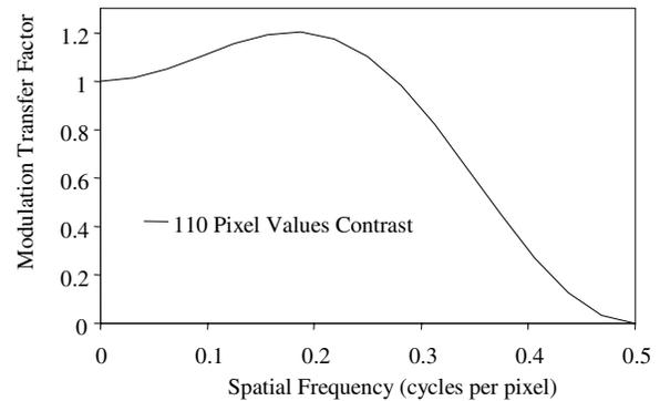
Figure 3. MTF of a system with a linear sharpening filter.
