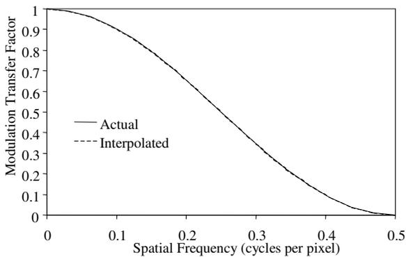
Figure 6. The result of applying regression to the curves in Figure 5 in order to estimate the 'linear' component of the MTF.
