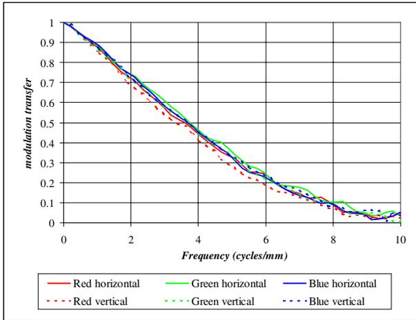
Figure 8a. Bi-directional color MTFs for a color sequential array scanner - registration correction OFF
