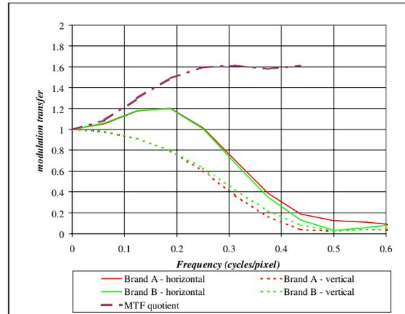
Figure 9. Bi-directional luminance MTFs for 2 differently branded 2-megapixel cameras
