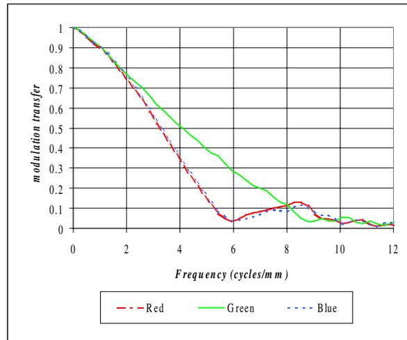
Figure 7. 300 ppi slow scan MTFs for a linear array scanner showing no color misregistration.
