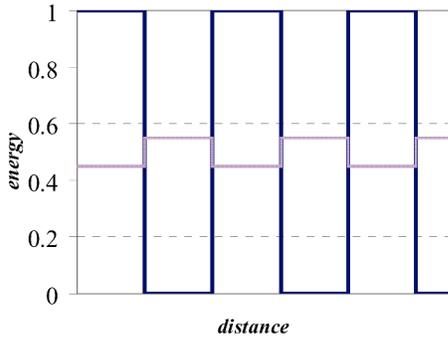
Figure 1. Idealized sampling and modulation loss for rectangular line spread function
