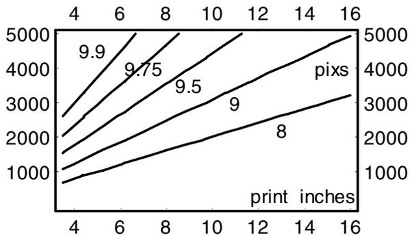
Figure 1. Relationship between number of sensor x-pixels and print x-dimension in order to conform to the range of sharpness values typical for analog photography.
