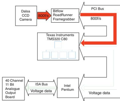
Figure 5. Schematic of control system
