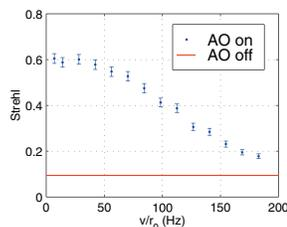
Figure 8. Strehl ratio as a function of the "wind speed" parameter  $v/r_0$  for  $D/r_0 \approx 5$ . (from Ref [6])
