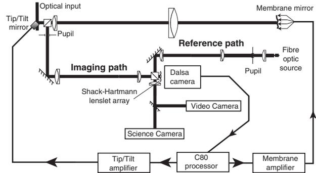
Figure 4. Schematic diagram of a breadboard layout for a low cost adaptive optics system.
