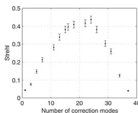
Figure 7. Strehl ratio as a function of the number of modes used in the control loop. (from Ref [6])
