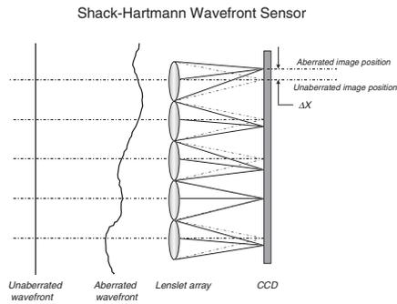
Figure 2. The Shack-Hartmann wavefront sensor.
