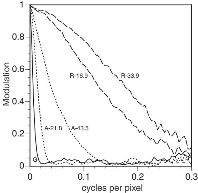
Figure 2. Modulation transfer function results: 43.5 and 21.8 micron AYAT films (dotted lines), 33.9 and 16.9 micron Regalrez films (dashed lines), and ground glass (solid line).
