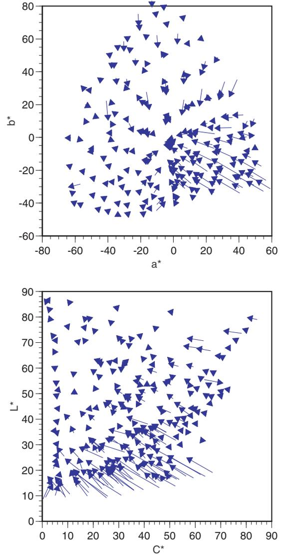
Figure 3. Vector plots for the 21.8 micron AYAT film applied to ground glass compared with clear glass
