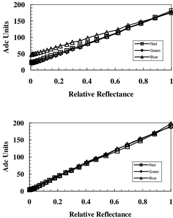
Figure 5. Dynamic range – top plot shows initial range for as-captured color images while the bottom plot shows range for color corrected images.
