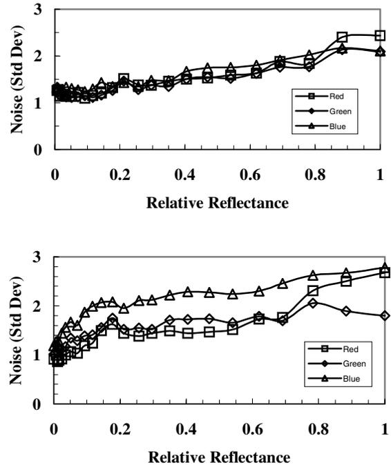
Figure 6. Temporal noise – top plot shows initial noise figure for as-captured color images while the bottom plot shows noise for color corrected images.
