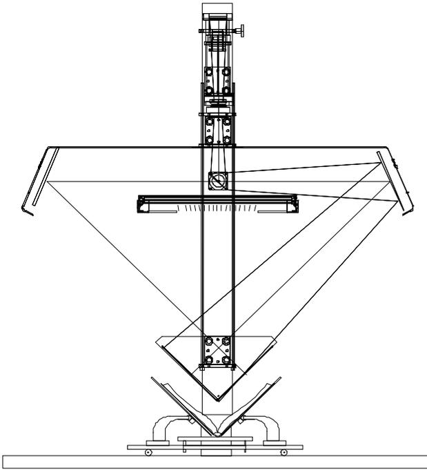
Figure 2. Bookscanner optical/mechanical design
