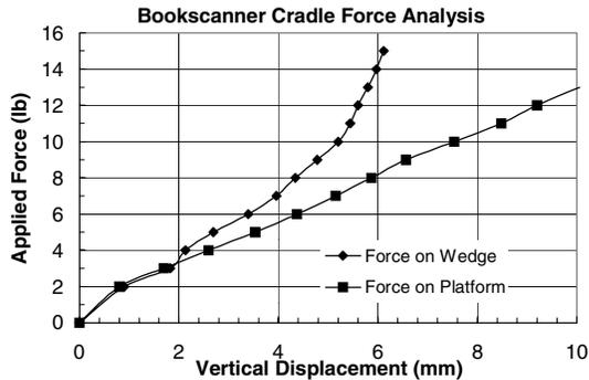
Figure 4. Applied force versus vertical displacement of the spring-loaded platform. The difference between the force applied to the platform alone versus the force applied to the wedge, through the book and to the platform is the additional force directed normal to the book pages
