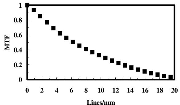
Figure 4. Modulation transfer function for the system optics
