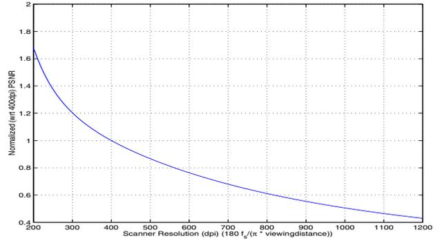
Figure 4. Overall relative VSNR (wrt 400dpi) as a function of scanner resolution.
