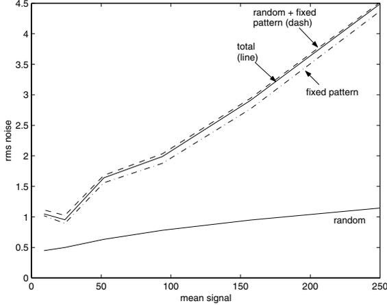
Figure 2. Component noise analysis for desktop scanner
