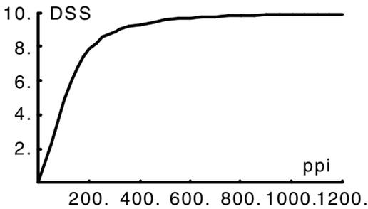
Figure 2. Digital sharpness as a function of pixels-per-inch in the digital printing device.
