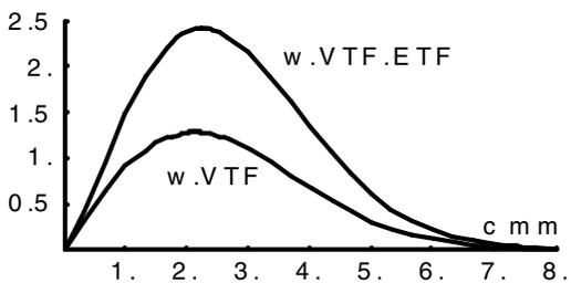
Figure 4. The image-detail spatial-frequency spectrum before and after cascading with the enhancement transfer function.
