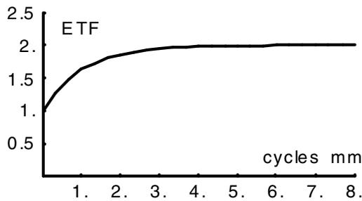
Figure 3. Enhancement transfer function associated with interlayer coupling mechanisms in silver-halide photography.
