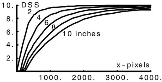
Figure 1. Digital sharpness as a function of required print size and number of detector pixels on a side.
