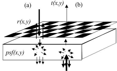
Figure 1. Schematic Diagram of (a) reflectance and (b) transmittance from a halftone image.
