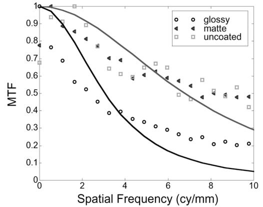
Figure 9. MTF paper measure from glossy coated, matte-coated and uncoated paper. The solid and dash lines are MTFs calculated from model in Eq. 8. with  $d = 0.039$  and  $0.016$  respectively.
