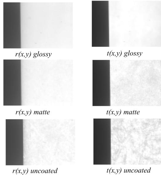
Figure 3.  $r(x,y)$  and  $t(x,y)$  of sharp edge contact on glossy, matte and uncoated paper.
