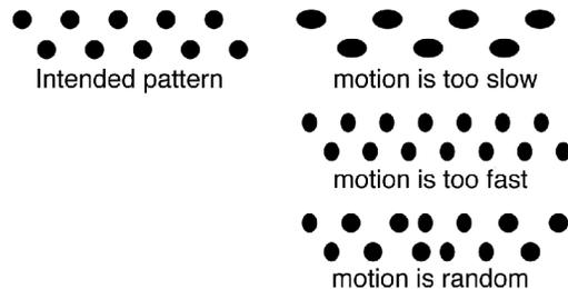
Figure 5: Dot Aspect Ratio and Spacing Deformation Due to Inadequate Motion Control
