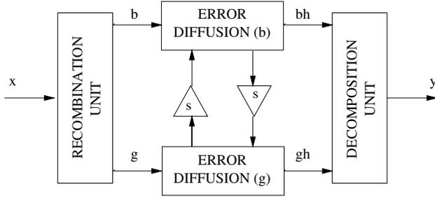
Figure 3: New Multitoning Algorithm based on gray level separation.
