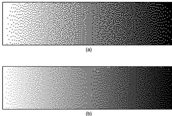
Figure 1: Halftoned gray scale ramp (a) binary (b) trilevel. Banding can clearly be seen in the ramp generated using trilevel error diffusion around gray level 0.5.
