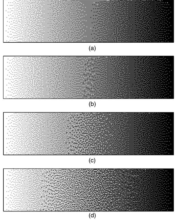
Figure 4: Gray Scale Ramps halftoned using the new multitoning technique with different conceivable gray level distributions.
