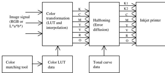
Figure 2. Signal flow of hi-fi printing
