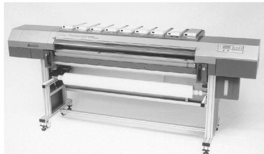
Figure 1. Textile inkjet printer Nassenger KS-1600 II
